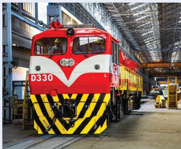
Customized made-in-India 3000 HP AC-AC cape gauge diesel electric locomotives for exports to Mozambique by RITES
